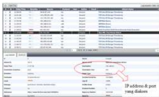
Gambar 4.10 Data serangan Open.SSL.Bleed.Attack
